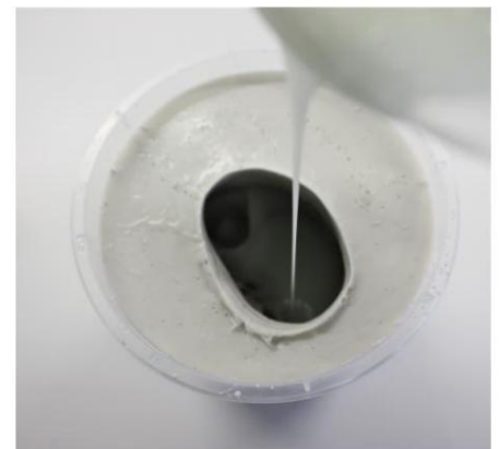
Fig. 5: The silicone is applied with a thin stream poured into the mold.
